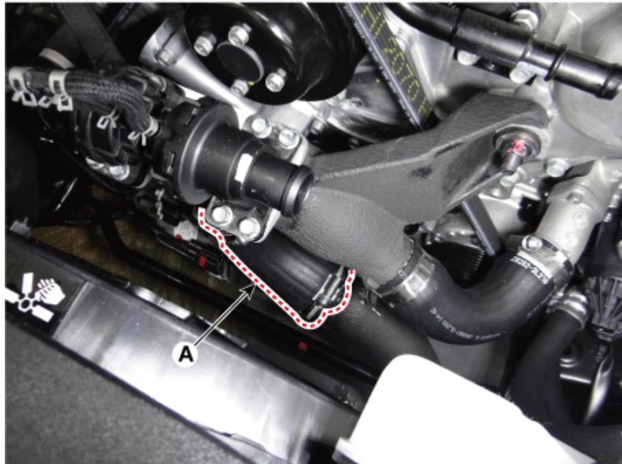
5. Disconnect the oil cooler water hose A (A).
